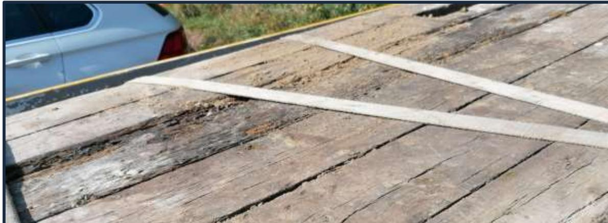
Photo of timber outrigger mats that were delivered to site with fungi attack clearly visible
