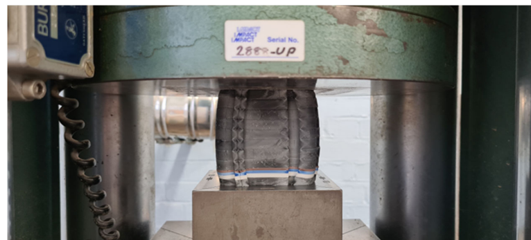
Figure 5: Photo of Test 8 | 100mm stack height under 230kN Load
