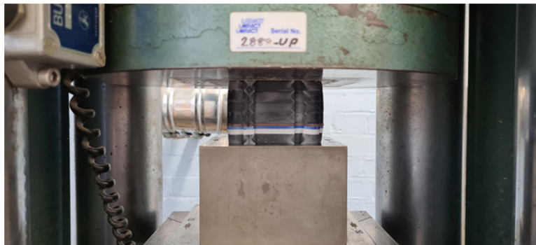
Figure 1: Photo of Test 4 | 60mm stack height under 230kN Load
