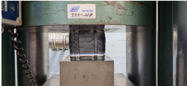
Figure 3: Photo of Test 6 | 80mm stack height under 230kN Load
