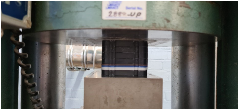
Figure 4: Photo of Test 7 | 80mm stack height under 143.8kN Load
