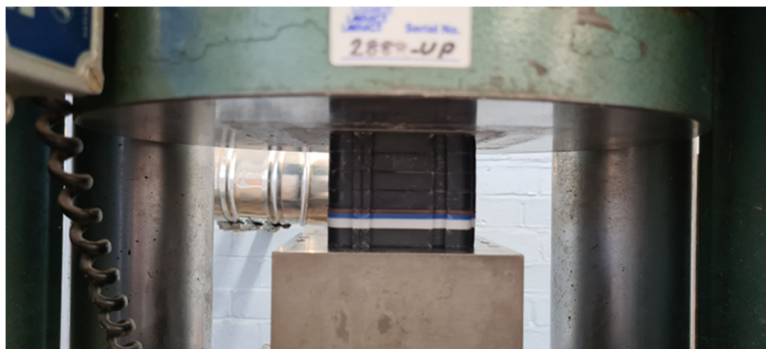
Figure 2: Photo of Test 5 | 60mm stack height under 143.8kN Load
